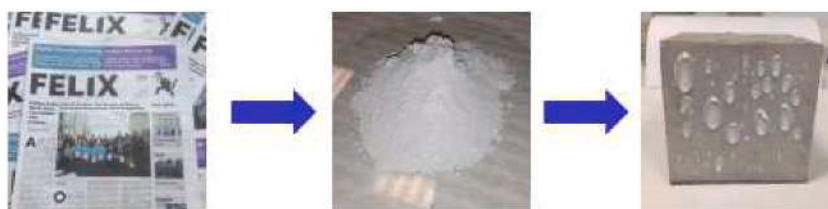
Fig. 7. Concept of turning waste newspaper into an admixture for producing hydrophobic concrete [9].
